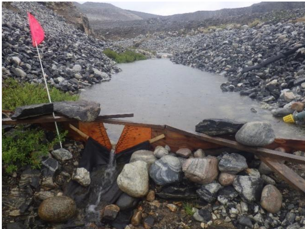
Photo 3.28 Graduated V-shaped weir in the outlet of Lake F3298
