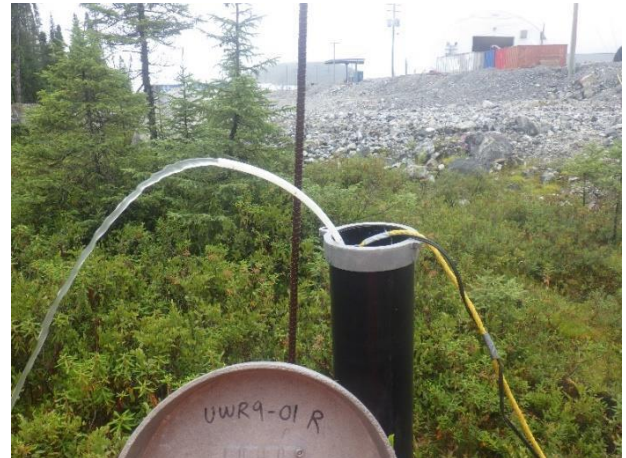
Photo 3.52 Sampling well UWP9-01R (July 31, 2021)
