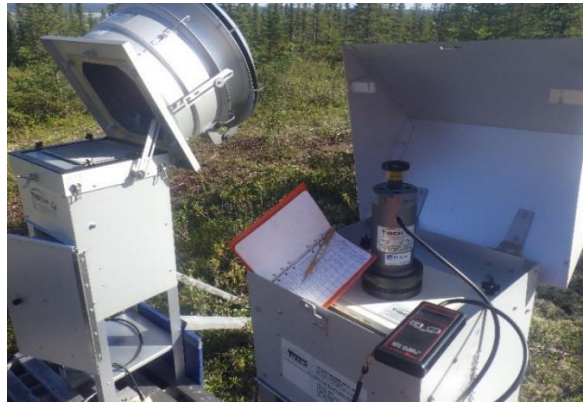
Photo 3.6 Installation of the sampling filter and calibration of the motor (August 23, 2021)
