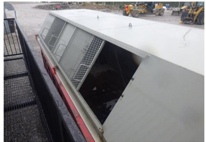
**Photo 3.42 Lids with sliding doors – dryhouse container**
