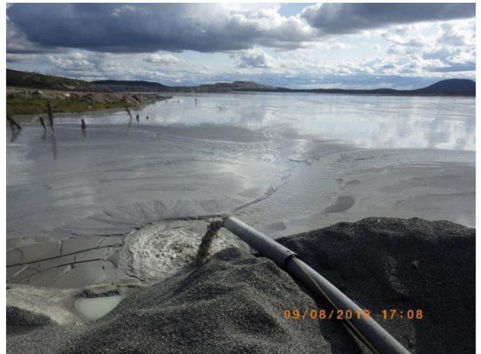
**Photo 3.58** Pool of fine processed kimberlite near a discharge point.
