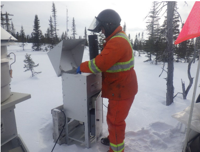
Photo 3.6 Installation of the air quality sampling filter (February 2020)
