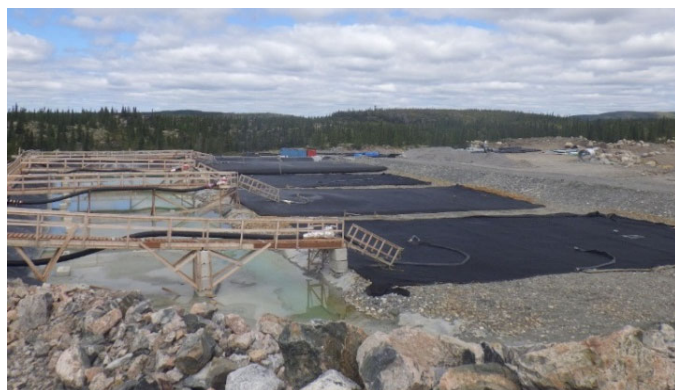
Photo 3.45 Modular treatment plant with Geotube® filter bags
